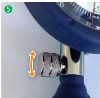
1. For use close the release valve by turning the knurled screw (Figure 5) and connect the cuff pressure monitor – where applicable with a connecting tube – to the pilot balloon of the tracheal cannula or the endotracheal tube. It has to be observed for all connections with a one-way-valve that the valve is opened, because with closed valve the cuff pressure will not be displayed correctly.
